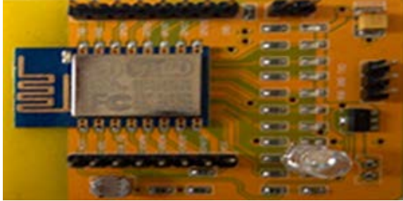
Figure 3. physical image of the WiFi module
